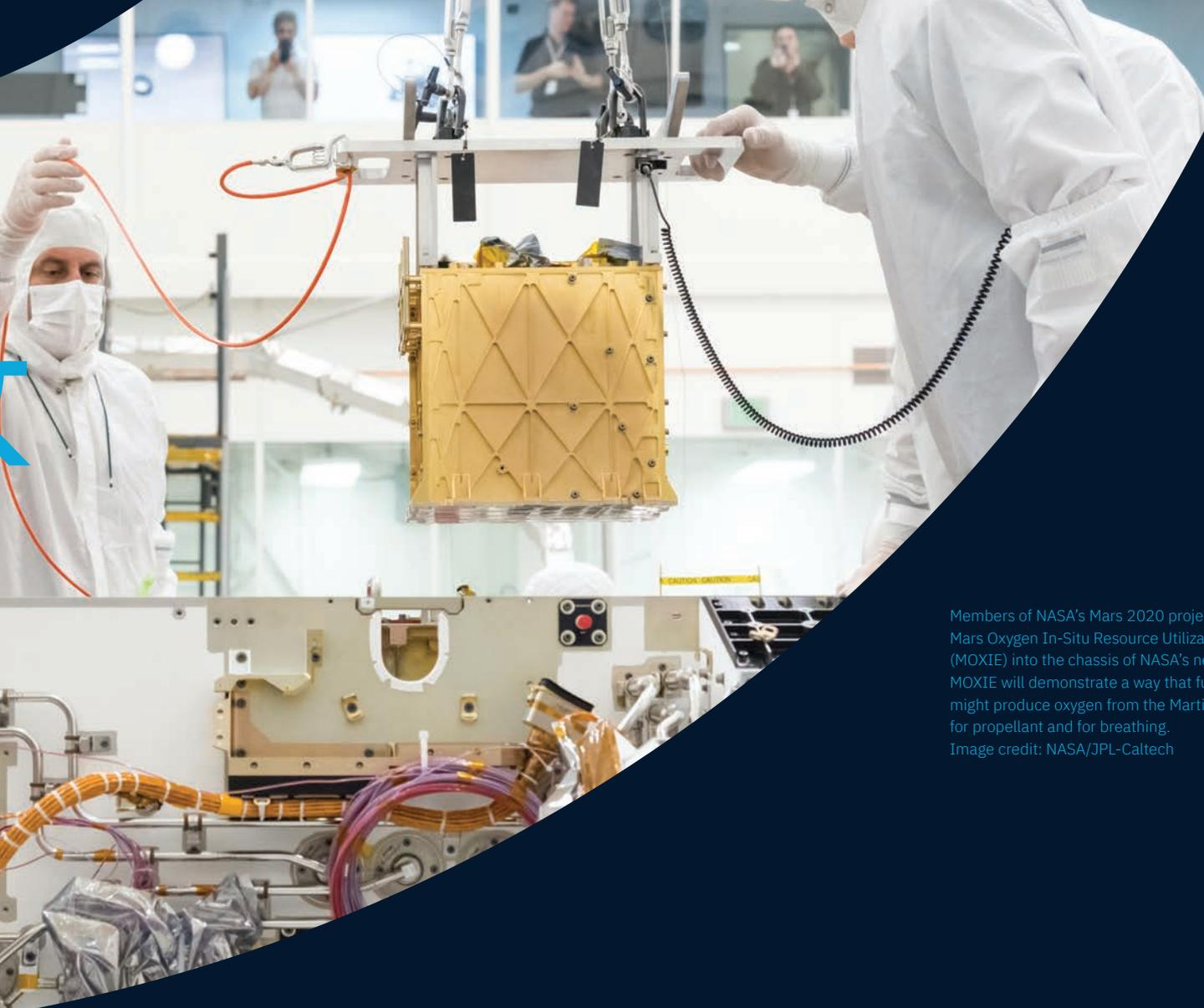
Members of NASA's Mars 2020 project install the Mars Oxygen In-Situ Resource Utilization Experiment (MOXIE) into the chassis of NASA's next Mars rover. MOXIE will demonstrate a way that future explorers might produce oxygen from the Martian atmosphere for propellant and for breathing. Image credit: NASA/JPL-Caltech
