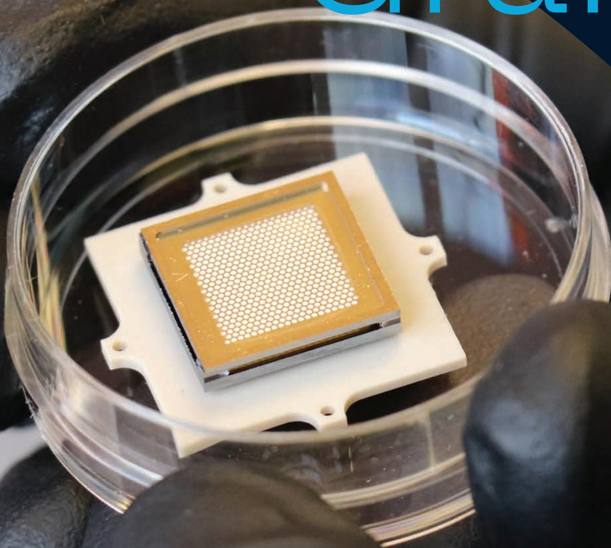
The Space Propulsion Laboratory engineers tiny, highly-efficient electro-spray spacecraft thrusters that improve the maneuverability of small satellites.
